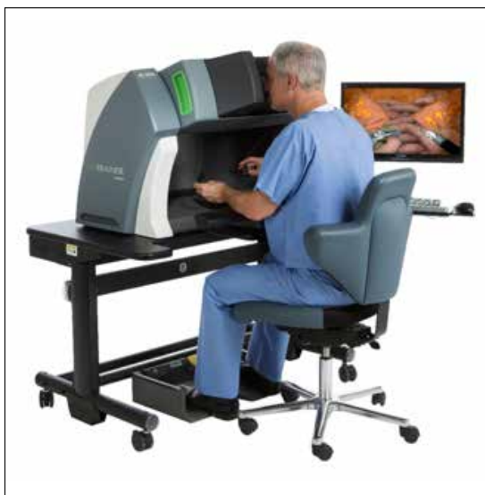
FIGURE 8 dV-Trainer simulator with MaestroAR (augmented reality)
