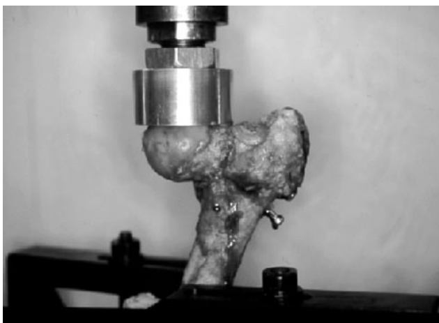
Figure 3. Representative inferior screw backout during mechanical testing of the vertically placed screws. Copyright 2007, Virak Tan, MD. Printed with permission.
