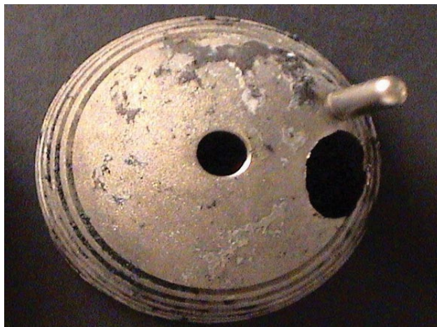
Figure 8. Worn-through shell. Retrieved acetabular component after revision for metallosis shows complete wear-through.
