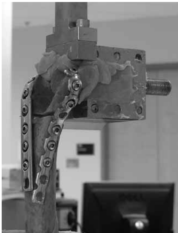
Figure 2. Torsional loading of 90° construct.
