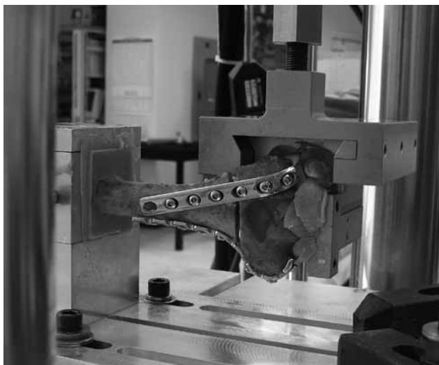
Figure 1. Mediolateral stiffness loading of 90° construct.
