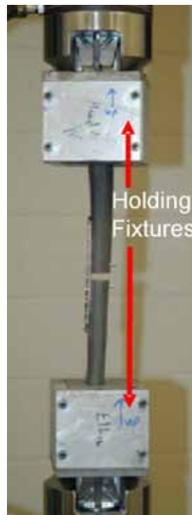
Figure 3. Experimental setup for external rotation torsion.
