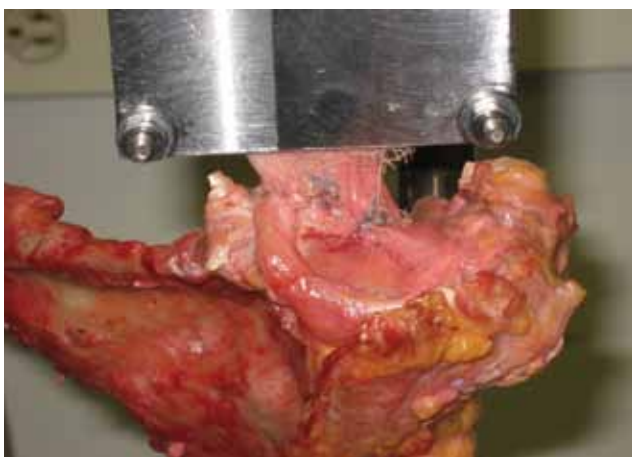
Figure. Jig for biomechanical testing loaded with scapula containing Bankart lesion repaired with knotted suture anchors. Custom sinusoidal clamp attaches directly to capsulolabral complex, allowing simultaneous testing of entire bony and soft-tissue repair.
