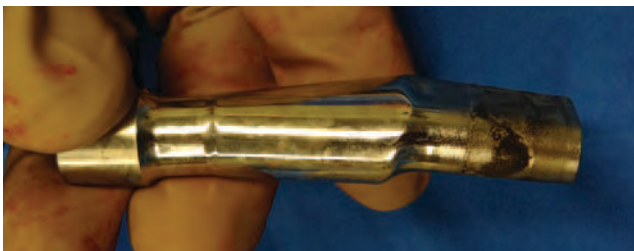
Figure 4. Intraoperative photograph of the corrosion material seen on the neck and femoral stem body junction after excision of the soft tissue mass.
