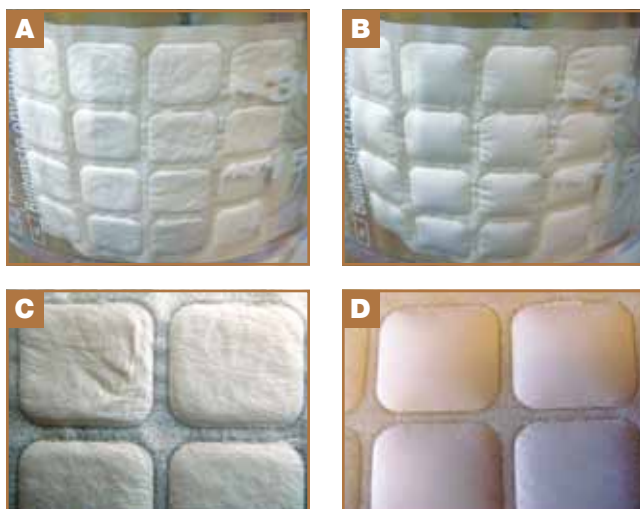
Figure 2. Cast liner in standard hospital wall-mounted bedside suction chamber at atmospheric pressure (A) and at full suction (B). Cast liner near sea level at major international airport (C) and at cruising altitude of 31,000 ft in a Boeing 757 (D). Note expanded volume of air cells.
