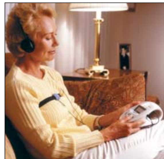
The RESPeRATE device uses melodic tones to progressively slow the patient's breathing.
