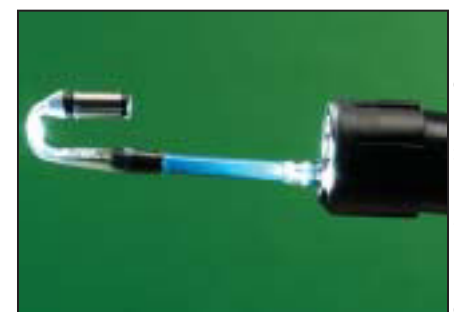
The retro-scope consists of a camera and light source on a flexible catheter.
