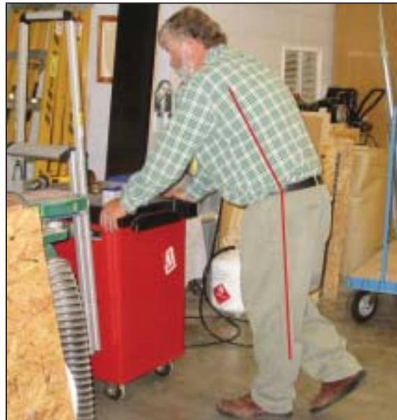
Before the height of this cart was modified, the user had to bend forward to push it around the workplace.
