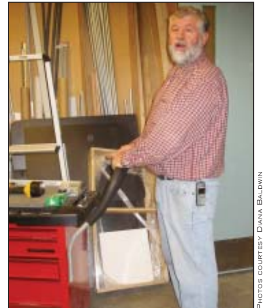
With a raised handle on the cart, the user can stand upright and move it more easily.
