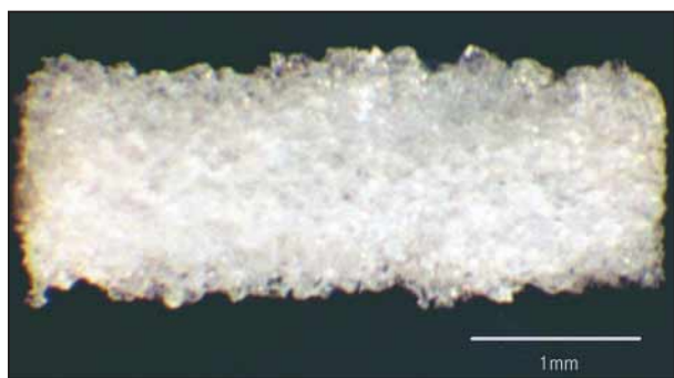
The matrix is porous and bioengineered to provide a scaffold for tissue in-growth and tube closure.
