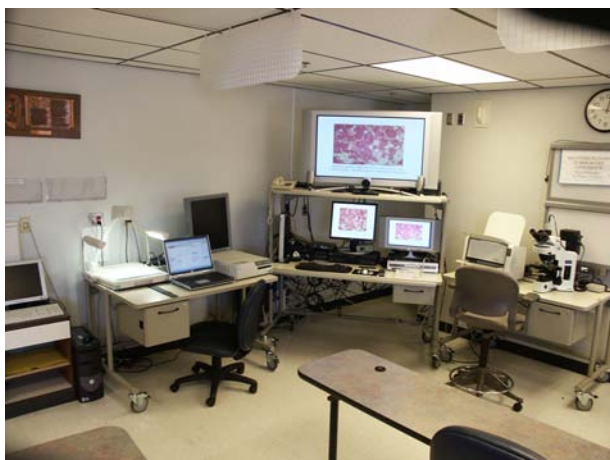
FIGURE 1 A view of the Telesynergy videoconferencing and medical consultation workstation at UPMC McKeesport. The main workstation for initiating control and distributing information contents during conferences is in the center (the two-tier desk with the large screen on the top). To the right is the station that is used for viewing microscopic images in real time and for downloading high resolution film based images with a dicom scanner. The desk to the immediate left of the 2-tier desk is has the equipment for retrieving electronic images (computed tomography, positron-emission tomography, magnetic resonance, sonography, etc) from local and distant medical sources. The equipment on the far left desk is used to link with web sites that are not linked to the main system computer and codec but provided through other secondary videoconferencing linkage so that video can be streamed (out and in).
