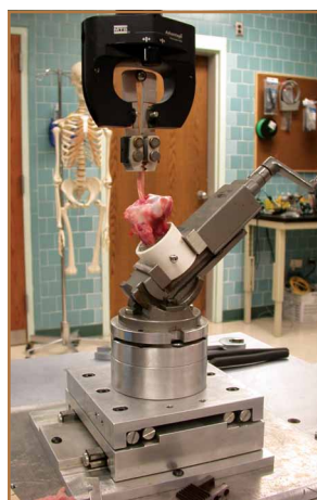
Figure 2. Test configuration for load tests. Load fixture used (top to bottom): pneumatic grips, custom pincer attachment, angled vise mounted to base with free-moving rotation and x-y stages for centering graft under load applicator. Tibial specimen after cyclic testing.
