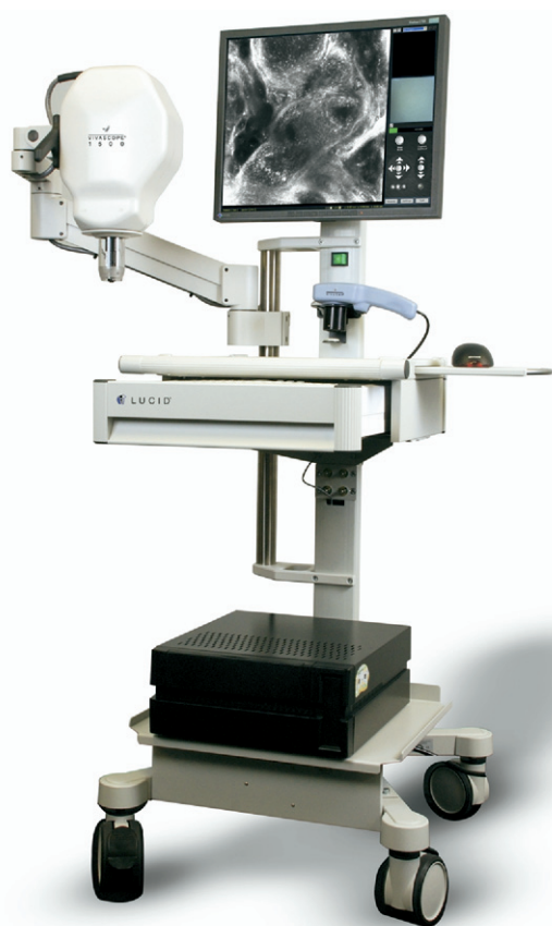
Figure 2 Confocal instrument: The VivaScope® 1500 is mounted on a cart with the VivaCam™ which produces dermatoscope-like wide field-of-view images. (Courtesy of Lucid, Inc. Rochester, NY). (Color version of figure is available online.)
