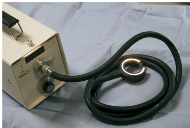
Figure 15 The Vein Lite (Wagner Medical) consists of the power source, a fiber optic cable, and a C-shaped light output. A dial on the power source allows for adjustment of the light output (up to 150 W).
