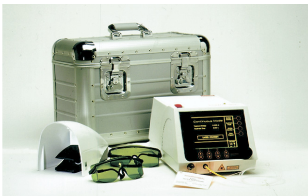
Figure 12 The laser set includes the laser console, foot pedal for laser activation, 2 pairs of protective eyewear, and a kit carrying case. The laser console has a touch screen with controls for choosing pulse or continuous laser function and wattage selection. The console also gives a running total of the energy administered to the vein being treated. Photo courtesy of Angiodynamics, Inc.
