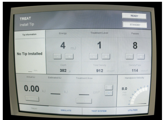
Figure 5 The treatment screen on the Fraxel Re:Store device allows the user to set the energy (depth) and treatment level (total density of treatment columns for the given number of passes). Total energy delivered is recorded on the lower left portion of the screen. Note that the device keeps track of the hand piece velocity on the lower right to alert the user if they are moving too fast for the device scanner to keep up.
