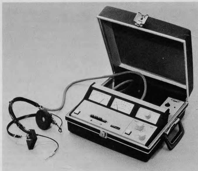
Madsen Portable Impedance Audiometer Model ZS75-1 (Courtesy of Madsen Electronics Canada Ltd., Oakville, Ontario)
