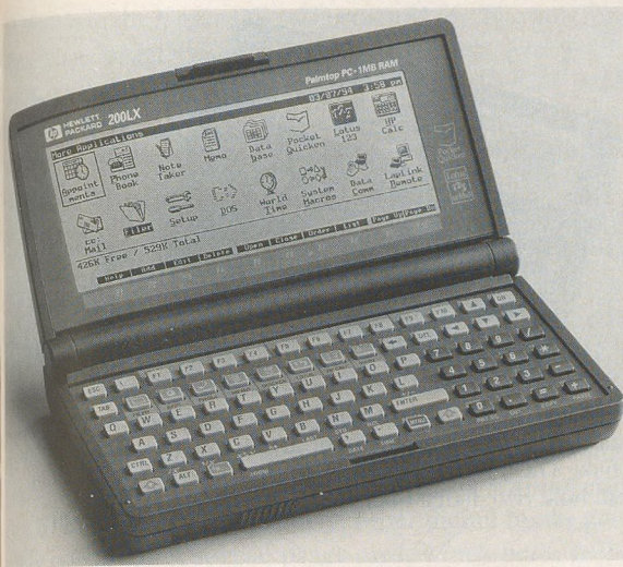
Figure 2. The Hewlett-Packard 200LX is a palmtop computer with miniature keyboard which uses the DOS operating system. It comes with a wide variety of useful software built in, weighs 10 oz, and measures 6.5×3.5×1 in. The HP 200LX's ability to run DOS programs is a significant strength.
