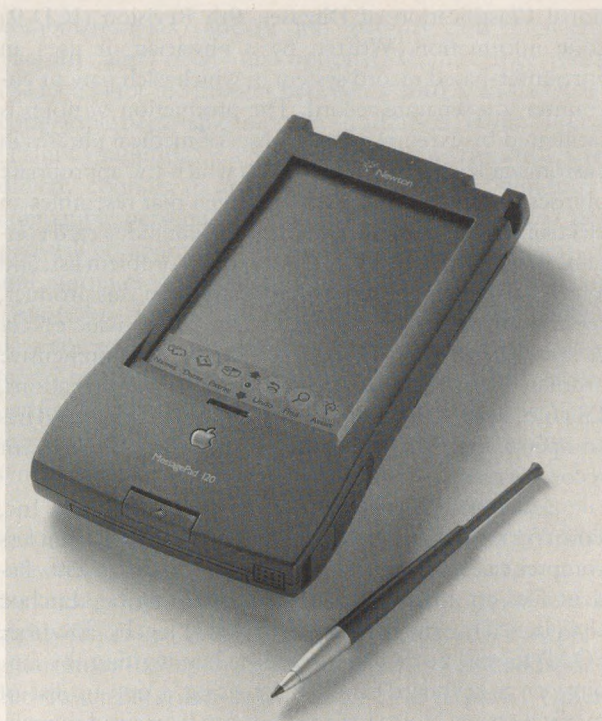
Figure 1. The Newton Message Pad 120 is a pen-based, hand-held computer from the Apple Corporation which incorporates handwriting recognition. It weighs 1 lb, and measures 8×4×1.2 in. The Newton has the widest variety of medical software available of any hand-held computer, including both commercial and "shareware" software.
